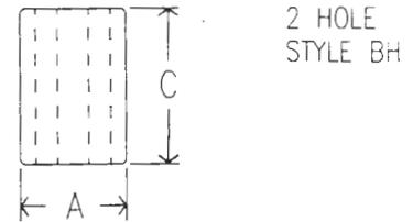
The BL style is the same as the BH with the addition of a winding slot along length "C" adjacent to both holes.
